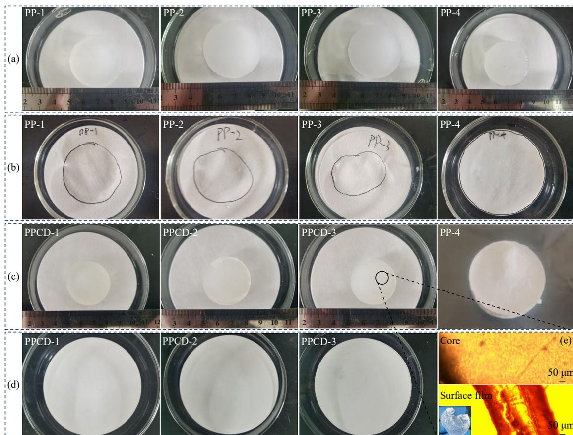
**Fig. 1** Photographs of PP hydrogels (a), filter papers below hydrogels (b), PPCD hydrogel FMPCMs (c), filter papers below PPCD hydrogel FSPCMs (d) and the optical microscope images of the core and the section of the surface film of PPCD-3 (e).
